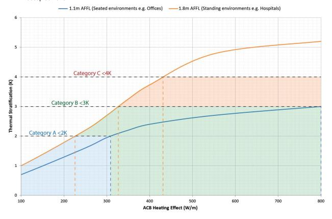
Note: The above relationships have been based on extensive Compact and Eco active chilled beam heating tests based on a worst case scenario I.e. Full height low surface temperature glazing and steady state conditions with no mixing of room air which simulates an unoccupied building.
